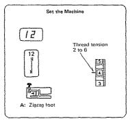
For general sewing, the lock-a-matic stitch is the tastest way to sew and secure a seam.
